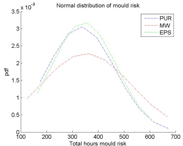
Fig. 7. Decision instrument: normal distributions of total hours of mould risk for different insulation types
