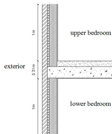
Fig. 1. Old brick wall with cavity
