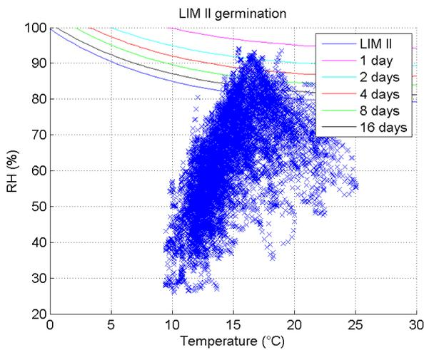
Fig. 5. Isoleth with coupled temperatures and relative humidities as calculated for one of the Monte Carlo runs (6cm PUR)
