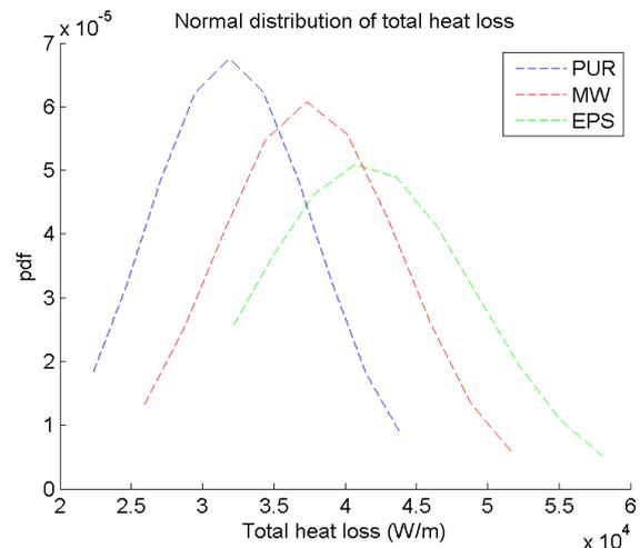
Fig. 6. Decision instrument: normal distributions of total heat loss for different insulation types
