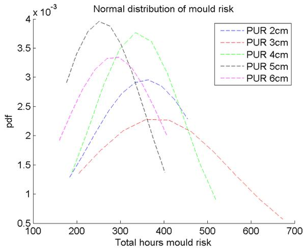
Fig. 8. Decision instrument: normal distributions of total hours of mould risk for different thicknesses of PUR
